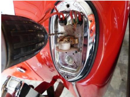
Hasbro Lite Brites my brother and I had when growing up. You start by removing the rear lenses and gaskets. New gaskets are included. The original bulb holders are riveted to the light housings and the two rivets need to be drilled out. They made this sound a little complicated, but 50 years of corrosion on old soft metal and it was easy enough. These are then discarded and the existing wires pulled
